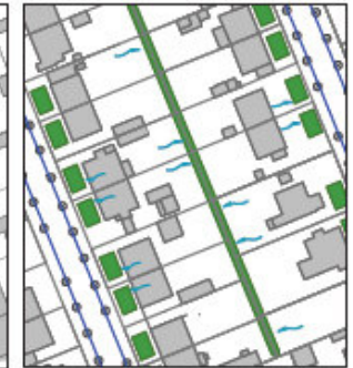
Fig. 44. The SUDS is placed in the backyard of the building block, receiving stormwater from all directions. Needs approval from all the stakeholders. Every household could also have their own SUDS in the front yard, capable of coping with the stormwater from the roof. Overflow is allowed to the street.
