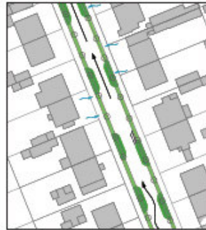
Fig. 40. SUDS elements are placed on both sides on the street either alternately or face-to-face. As the road is notably narrowed, it slows down the traffic. Placing the SUDS elements alternately, makes the street look curvy, whereas the face-to-face version leaves the street straight. Angle parking might be possible.
