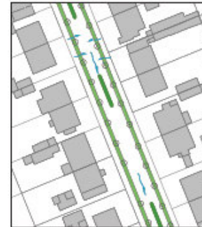
Fig. 43. The stormwater is lead in the SUDS that is placed in the middle of the road. In that case, the SUDS elements function also as a speed control. However, that kind of design could be suitable for wider roads and boulevards.
