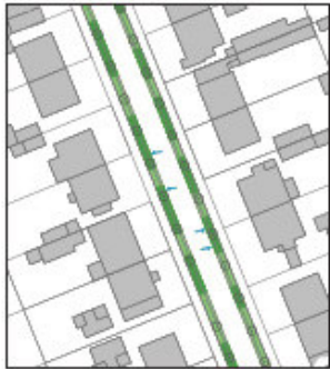
Fig. 39. The road is narrowed a little, to make room for the SUDS elements on both sides of the street. The width of the SUDS elements is the same along the road; therefore the overall image of the street is not altered much. The size of the SUDS elements might be too narrow for large amounts of stormwater.
