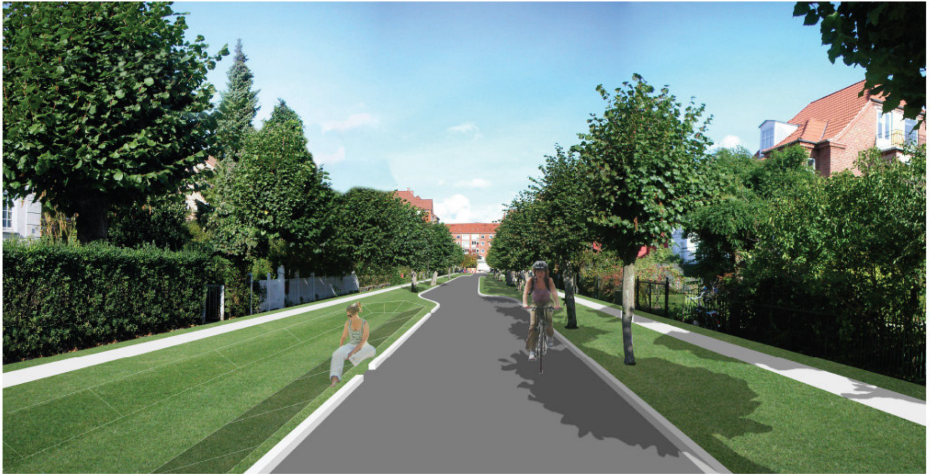
Illustration of the design: narrow, curvy road and green pocket with a wadi (curb cut for runoff inlet). In the background a green pocket for social events can be seen.
