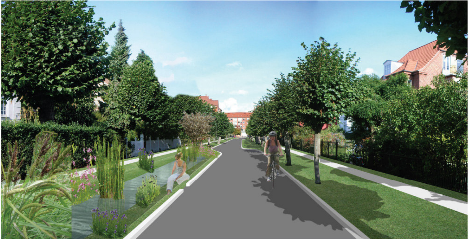
Illustration of the design with water and plants: narrow, curvy road and green pocket with a wadi (curb cut for runoff inlet). In the background a green pocket for social events can be seen.
