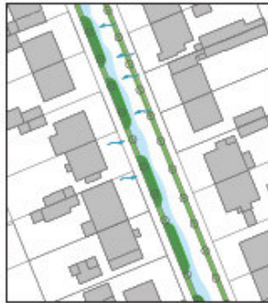
Fig. 41. SUDS elements are placed only on one side of the street, leaving the other side untouched. The road is also sloping on one side - in case of heavy rain, only half of the road would be flooded.
